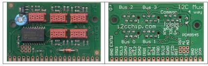
The 3.3V regulator in the top left corner could easily be replaced with a lower voltage one, or simple disconnected and the downstream VCC supplied by the low voltage slave device
