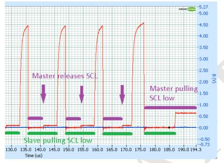
Here we see a slave (with weak outputs or series resistance), which clock stretches every clock pulse. In this case it is stretching SCL within the first 8 bits - the master releases SCL before the slave releases it. The small step in level makes it clear where the the master has released
