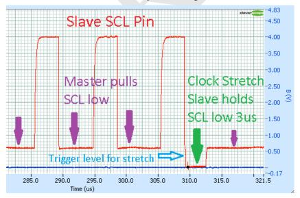
Attach the probe to the Slave side SCL. Here we see a Microchip PIC based slave stretching the clock for 3us after the ACK clock pulse. Note that the clock is not *actually* being stretched, as the master is still holding the bus low when the slave releases SCL.
