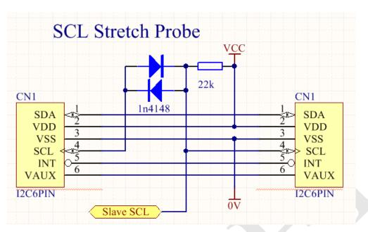
This is easily made on the small hub pcb that comes with the I2C Starter Kit or connector kits. Any diode will do, signal or power diodes.
